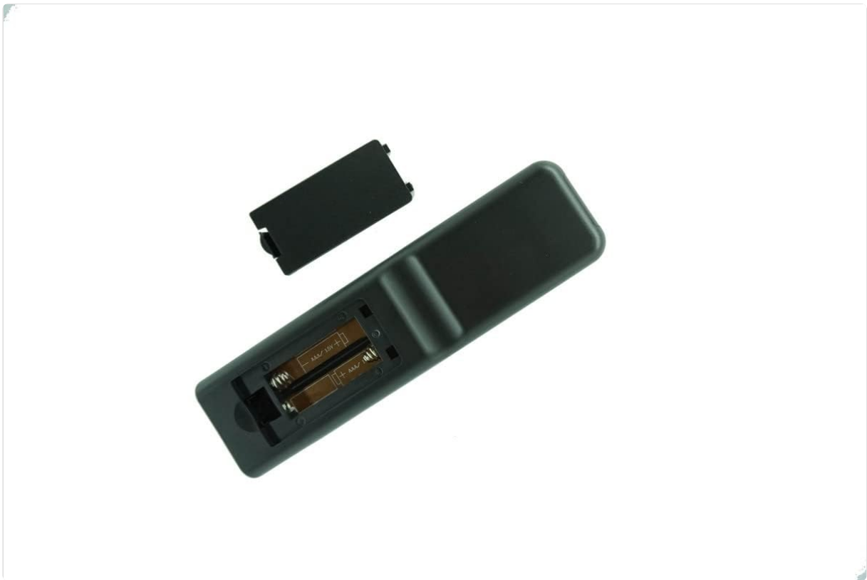
Figure 2: Back of the remote control with the battery cover removed, illustrating the correct orientation for AAA battery insertion.
