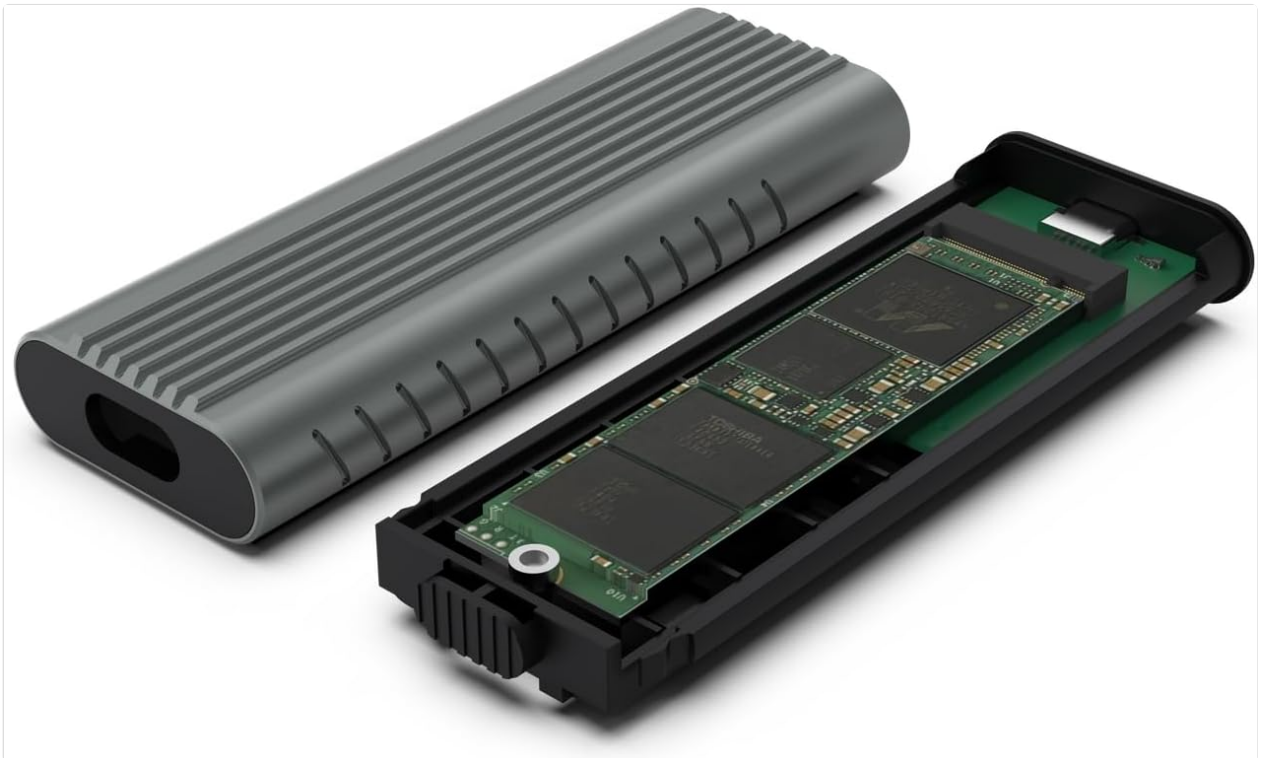
Image: The enclosure with an M.2 NVMe SSD correctly installed on the internal board.
