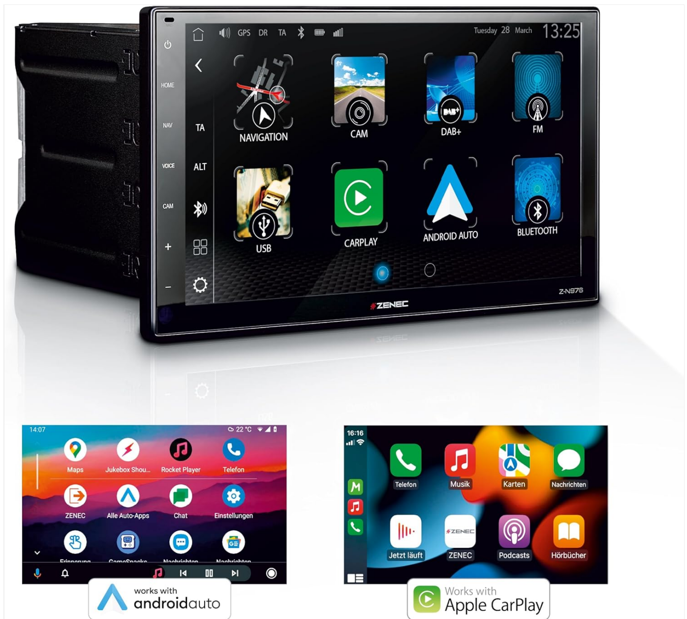
Figure 4.4: The Z-N976's main menu displaying icons for various functions including Navigation, Camera, DAB+, FM, USB, CarPlay, Android Auto, and Bluetooth, highlighting its comprehensive connectivity options.
