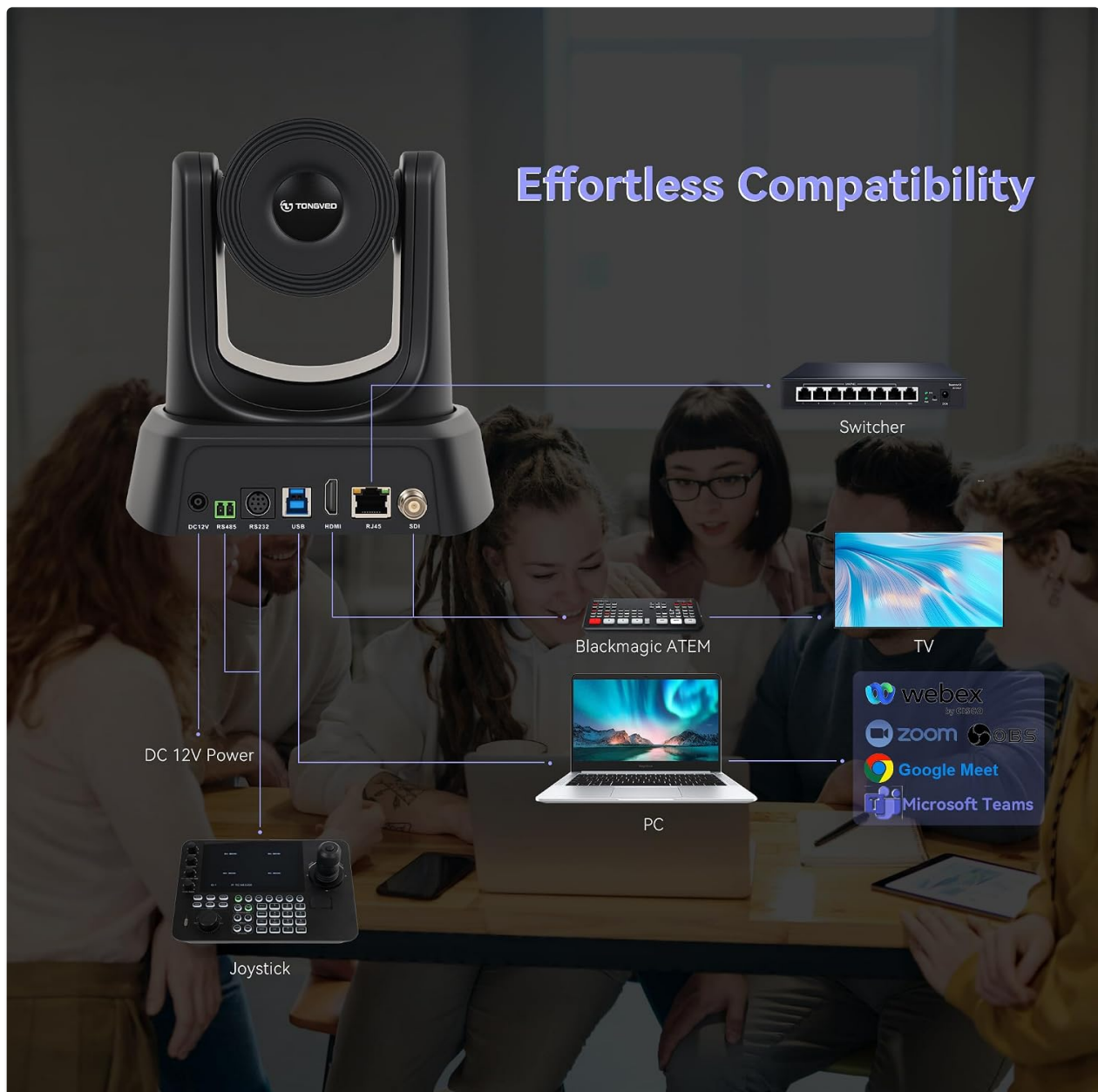
Figure 3.1: Rear panel connections of the TONGVEO PTZ Camera, illustrating various input/output options and compatible systems.
