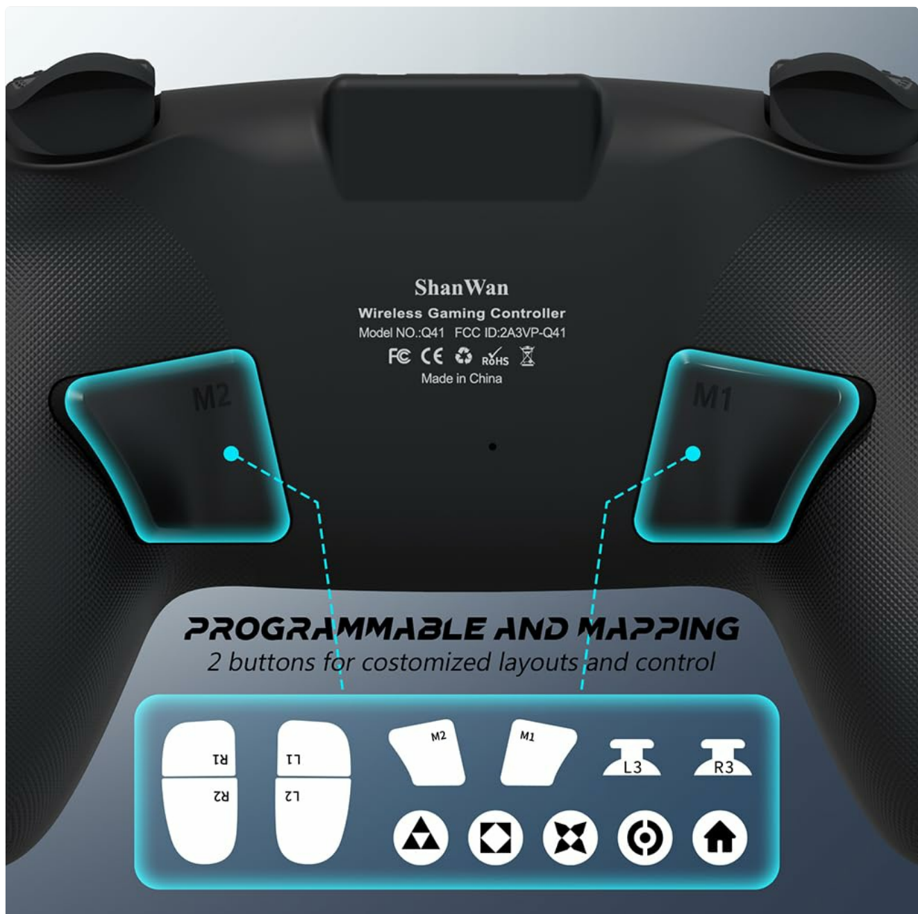
Image: The back of the ShanWan Wireless Controller, highlighting the M1 and M2 programmable buttons. An overlay illustrates various buttons (L1, R1, L2, R2, Triangle, Circle, Cross, Square, Home, L3, R3) that can be mapped to M1 and M2.
