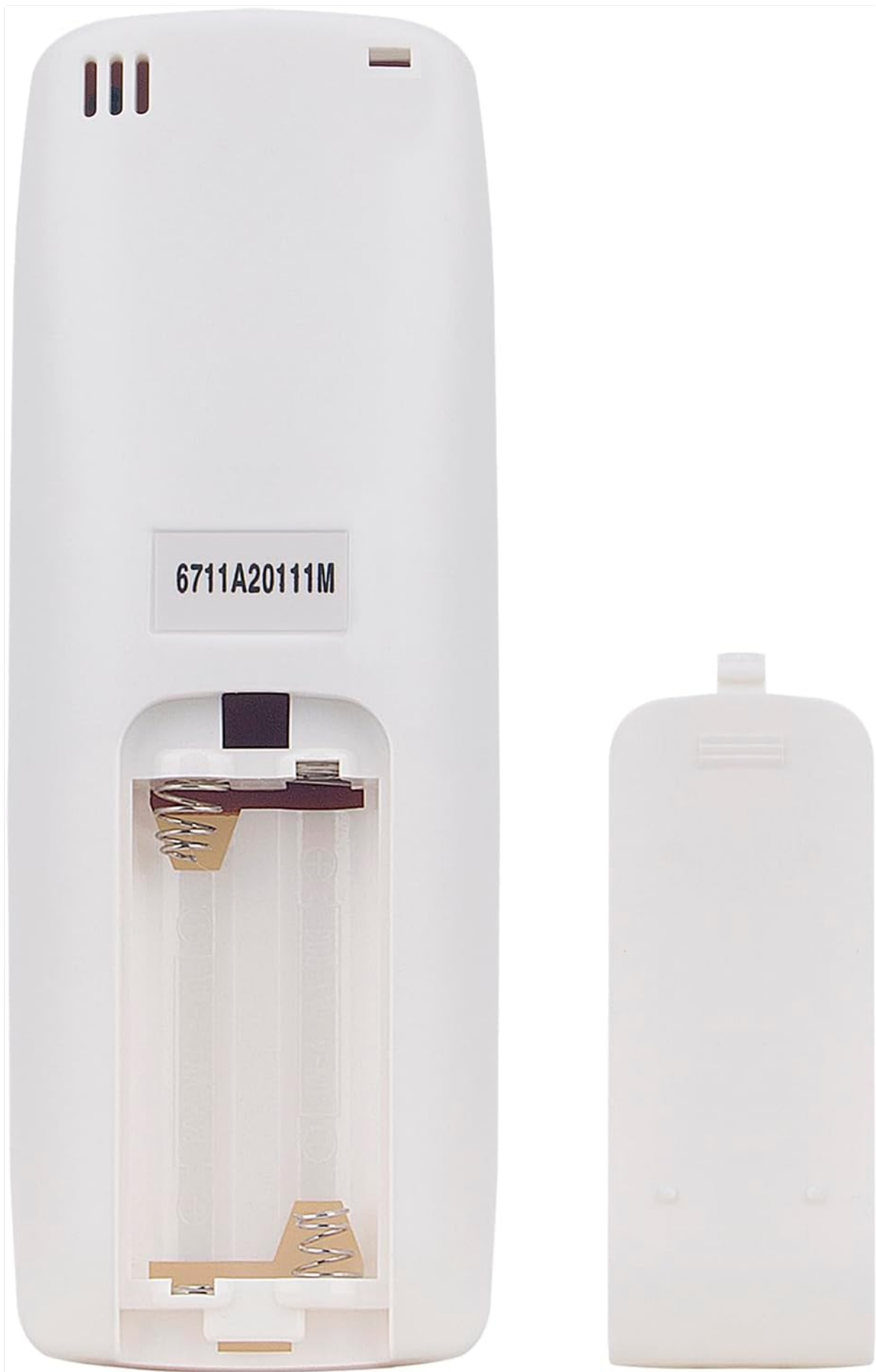
Image: Back view of the remote control with the battery compartment open, illustrating battery insertion.
