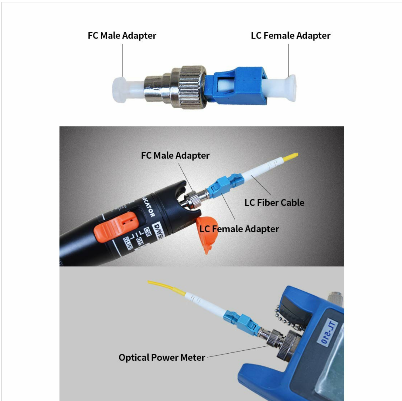
Image 6: Examples of the adapter in use, connecting an LC fiber cable to a Visual Fault Locator and an Optical Power Meter. The adapter is widely used in various applications:
