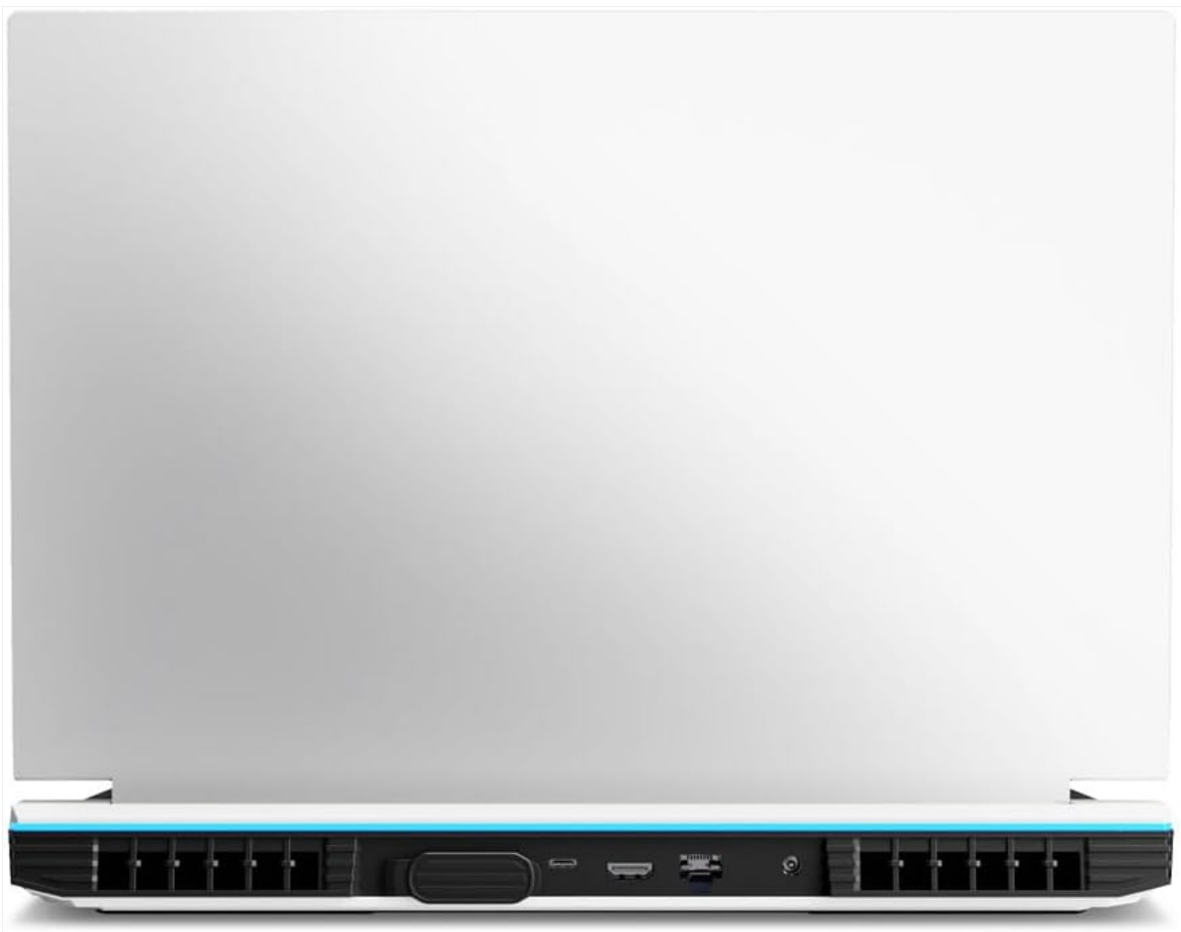
Figure 2.5: Rear view of the laptop, highlighting the HDMI, Thunderbolt, Ethernet ports, and cooling vents.
