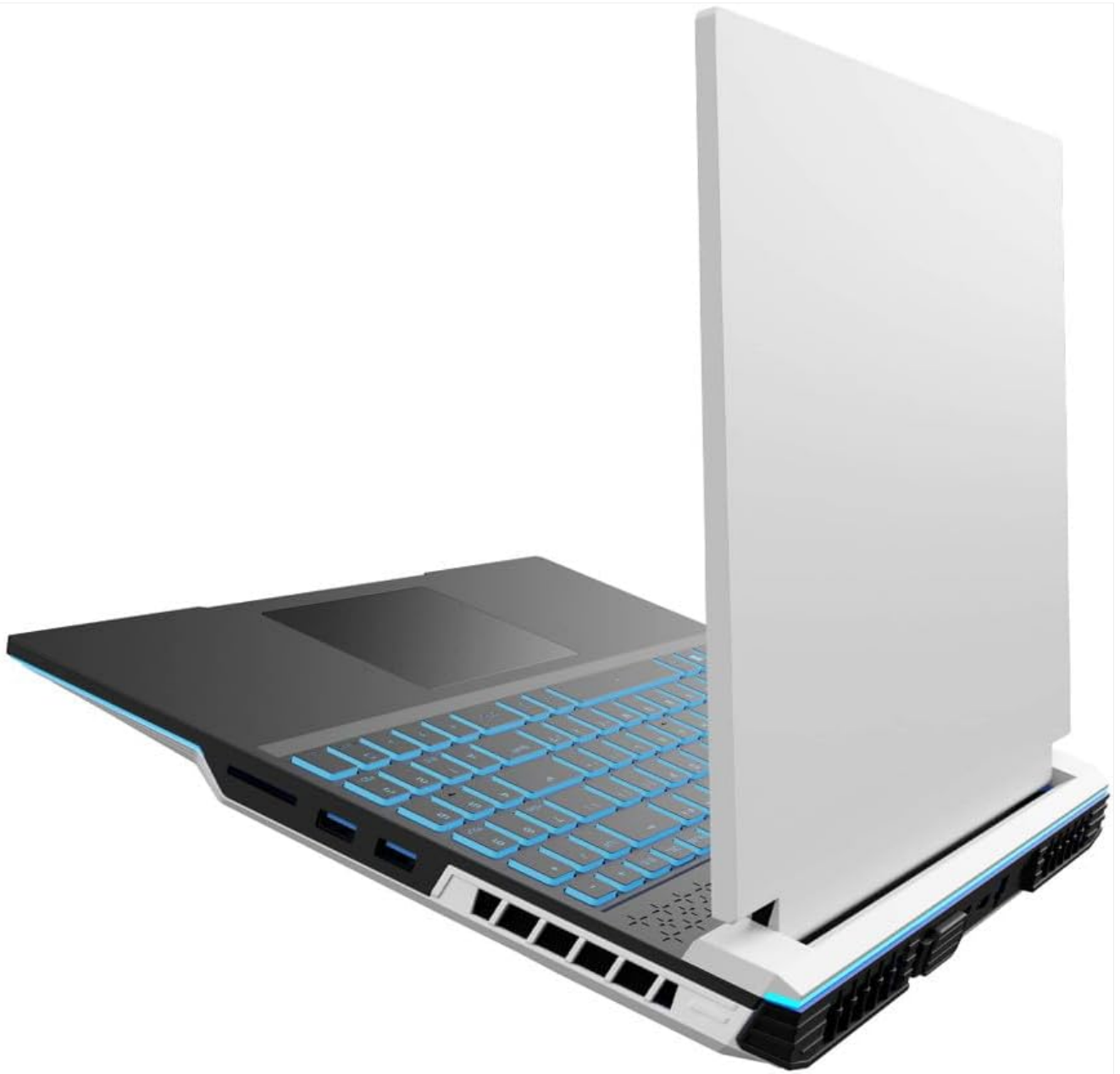
Figure 2.4: Right side view of the laptop, displaying additional USB ports and an SD card reader.
