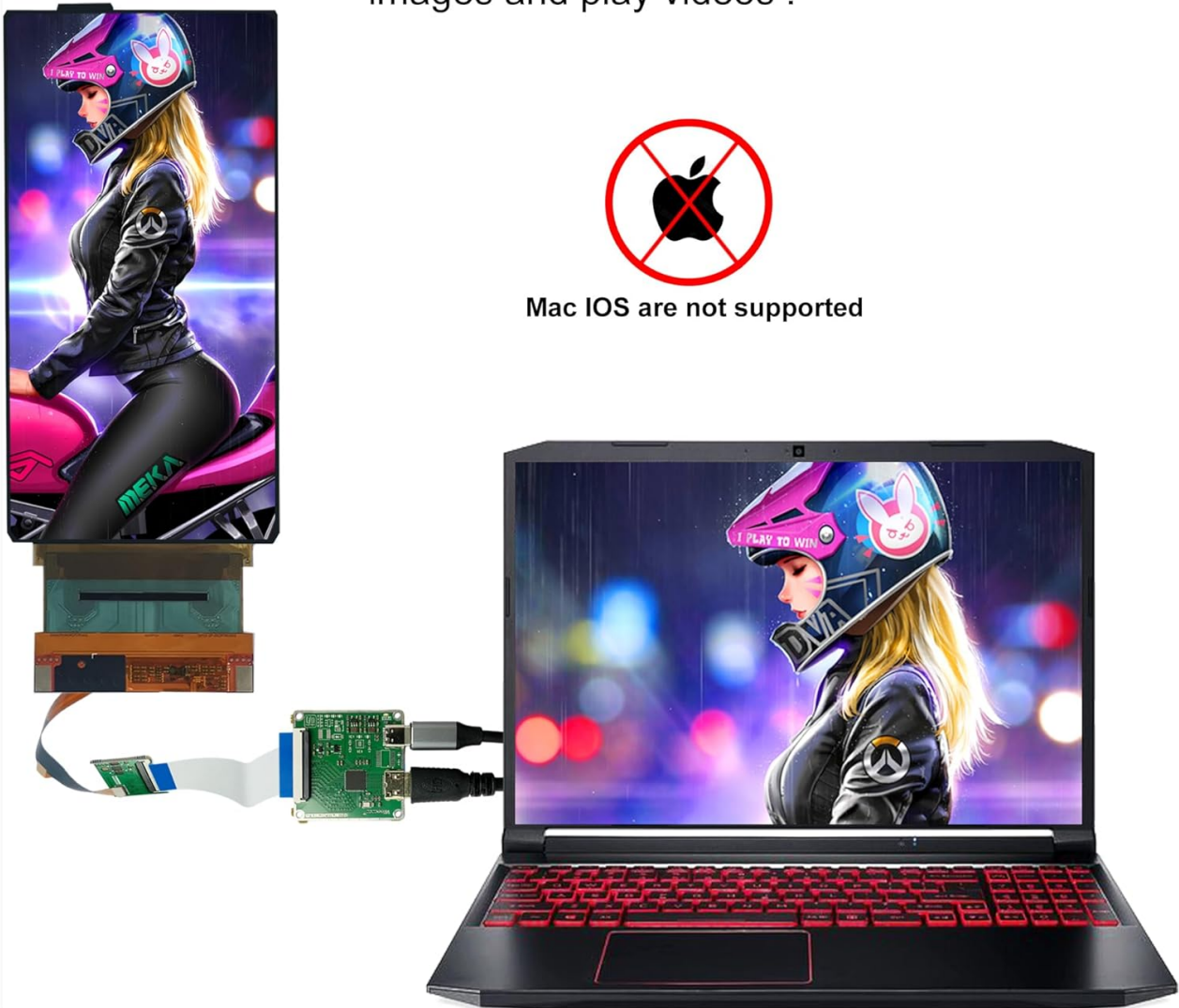
Figure 5: Connection diagram illustrating how to connect the flexible screen module to a Windows laptop. Mac iOS is not supported.
