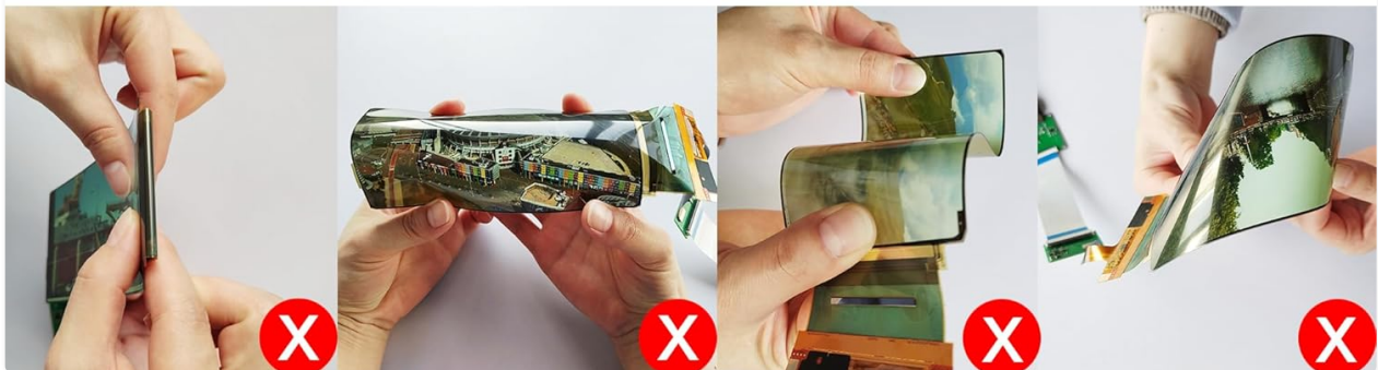
Figure 6: Guidelines for safely bending the flexible screen. Always handle with care and avoid prohibited bending methods to prevent damage.
