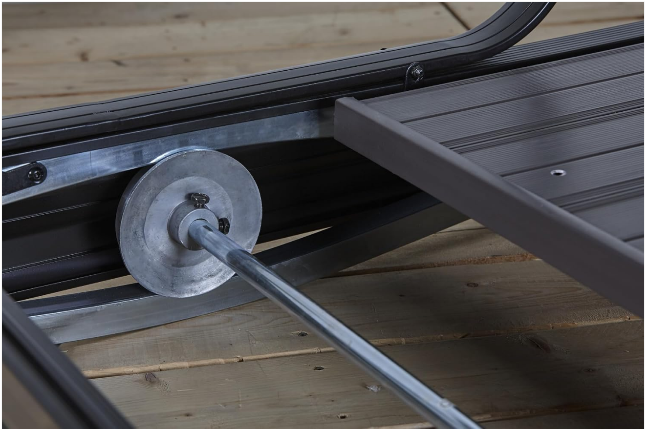
Figure 3: The wheel mechanism that enables the smooth gliding motion of the seats.
