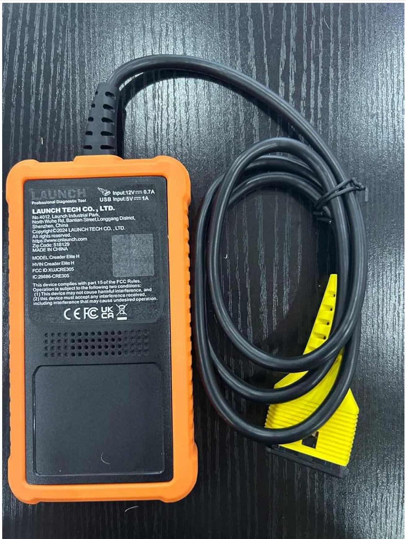
Figure 2.1: Rear view of the LAUNCH Creader Elite device. This image shows the back of the diagnostic tool, including its product label with model number and input specifications.
