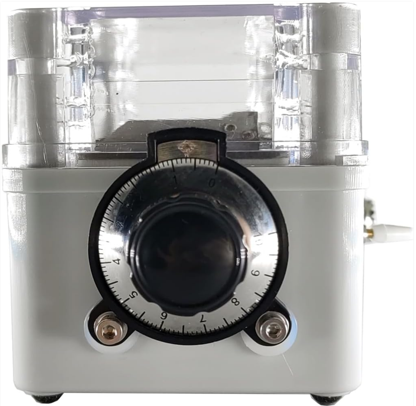
Figure 5.1: Front view of the MRA-821 main unit, showing the tuning knob used to adjust the antenna for optimal reception.
