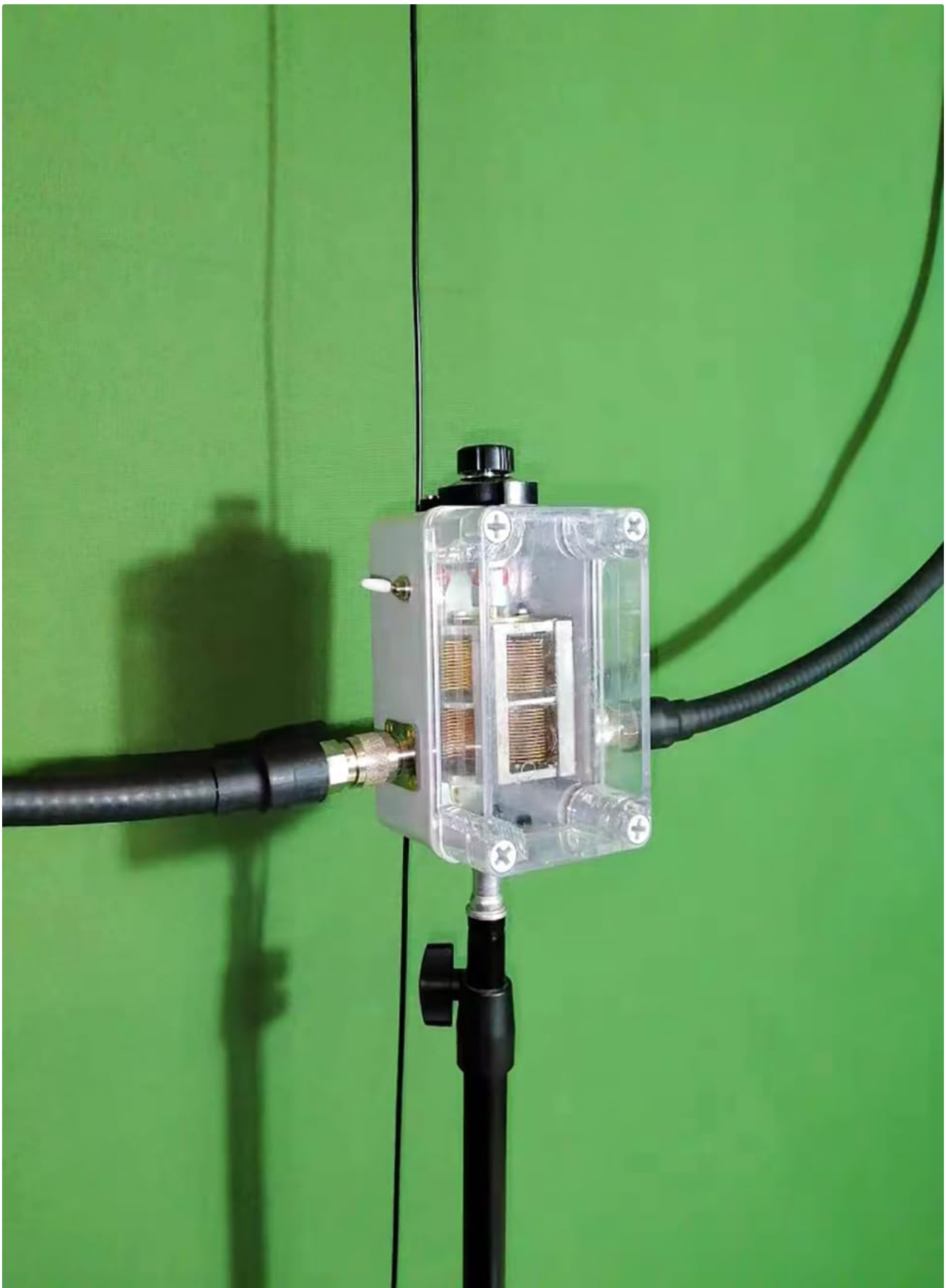
Figure 5.2: Side view of the MRA-821 main unit, showing the clear cover over internal components and the tuning knob on top.
