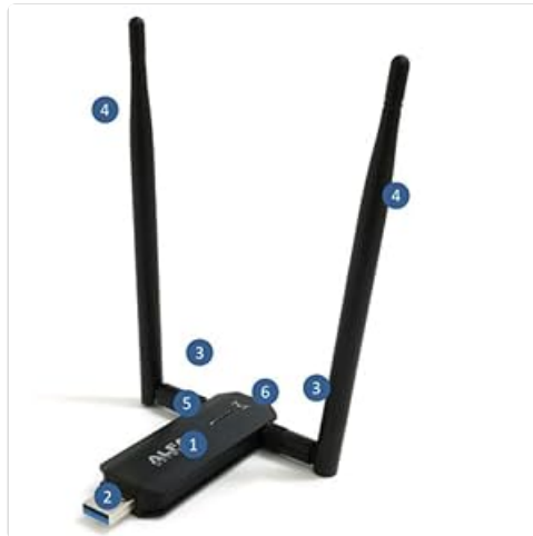
Figure 2: Components of the AWUS036AXM. This diagram highlights key parts of the adapter: 1. Main adapter body, 2. USB 3.0 connector, 3. Antenna ports, 4. Detachable antennas, 5. LED indicator, 6. ALFA Network branding.
