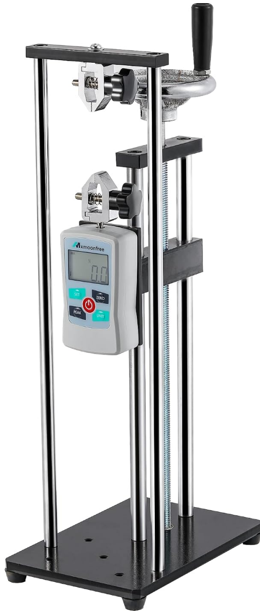
Figure 1.1: Assembled ZMF-500N Force Gauge and Manual Test Stand.
