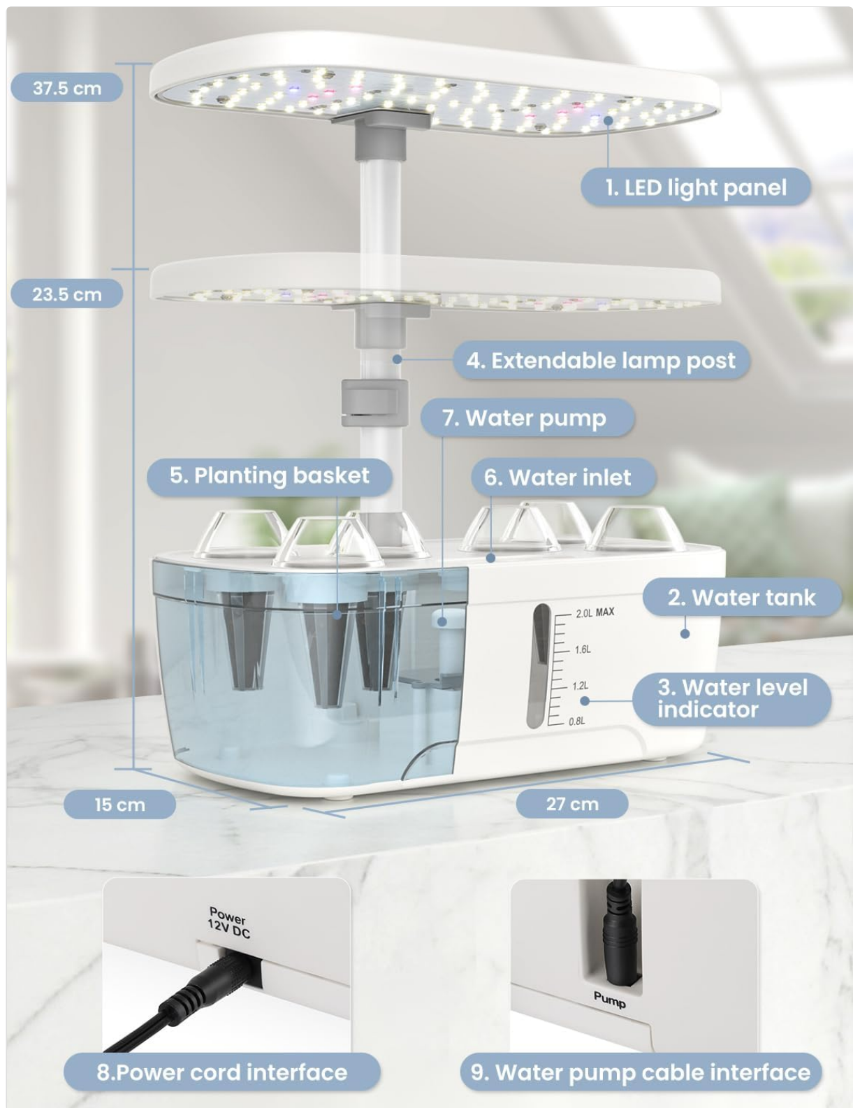
Detailed diagram showing the numbered components of the hydroponics system.
