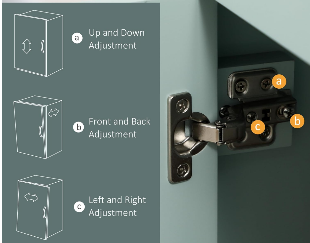
Image: Detail of an adjustable hinge, showing up and down, front and back, and left and right adjustment points.
