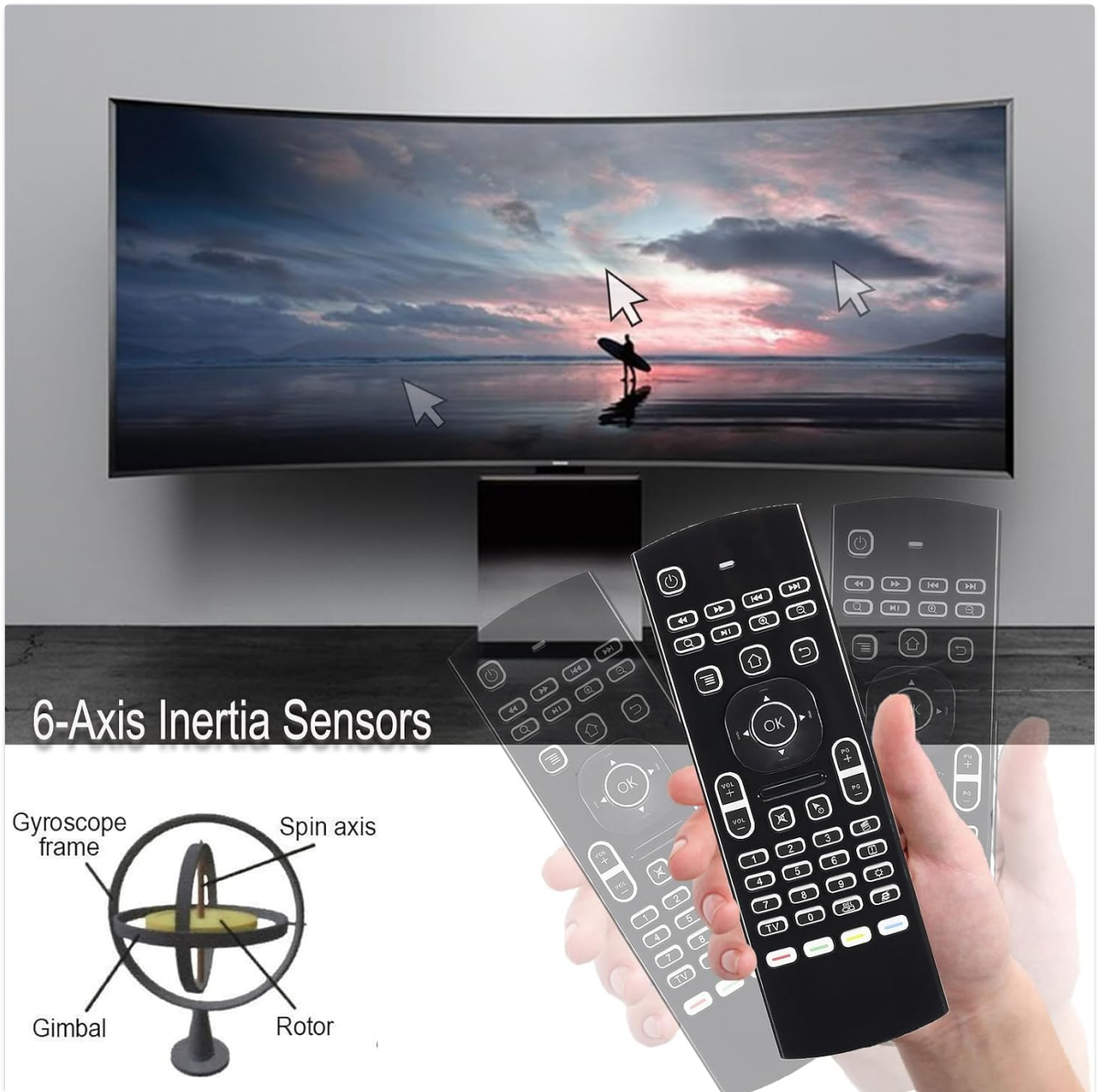
Image: The MX3 remote control being used as an air mouse, with a diagram illustrating the 6-Axis Inertia Sensors (Gyroscope frame, Spin axis, Gimbal, Rotor) that enable its motion-sensing capabilities.
