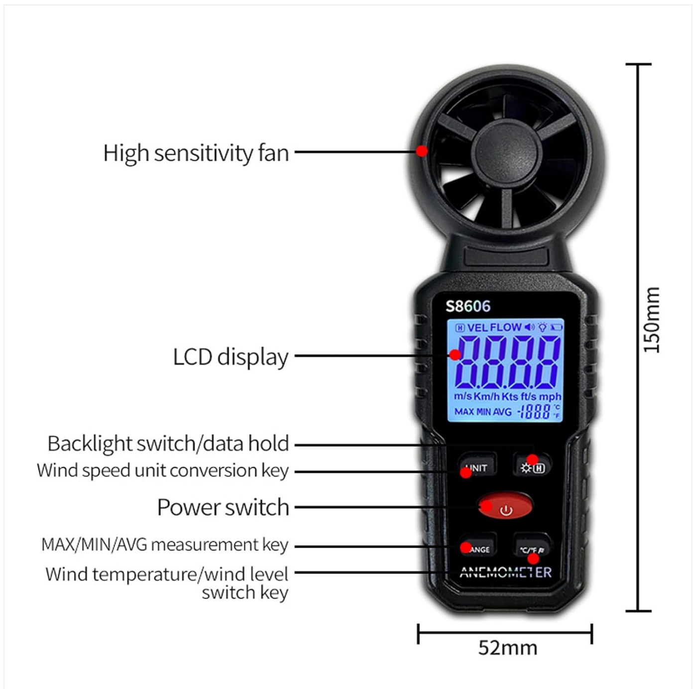
Figure 4.1: Front view of the S8606 Anemometer with key components labeled, including the high sensitivity fan, LCD display, and control buttons. Dimensions are approximately 150mm height and 52mm width.
