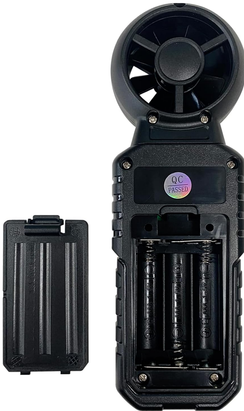
Figure 5.1: Battery compartment with batteries installed.
