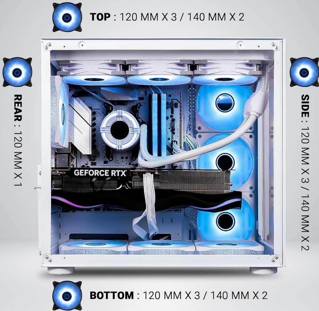
Figure 7: Multiple fan support locations.
