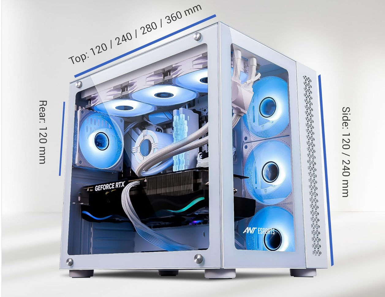
Figure 8: Large liquid cooling support options.
