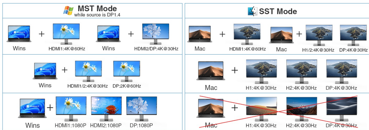
Figure 7: USB-C Port Compatibility. Compatible ports include Thunderbolt 3/4, USB-C with full function (DisplayPort, Data, Power Delivery), or USB-C with DisplayPort and Power Delivery. Ports that are 'Data only' or 'Charge only' are not compatible for full functionality.
