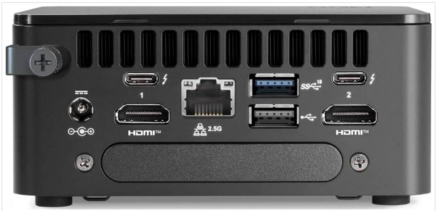
Rear view of the Intel NUC 13 Pro NUC13ANHi3, illustrating the power input, HDMI ports, Ethernet port, and USB ports.
