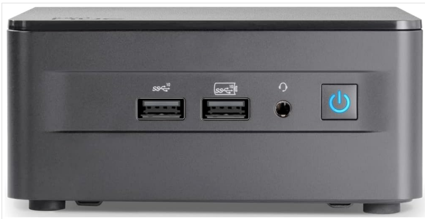
Front view of the Intel NUC 13 Pro NUC13ANHi3 Barebone System, showing USB ports, headphone jack, and power button.
