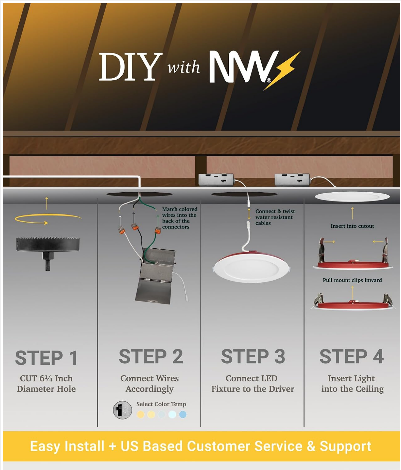
Image 6.1: Step-by-step visual guide for the canless installation process.
