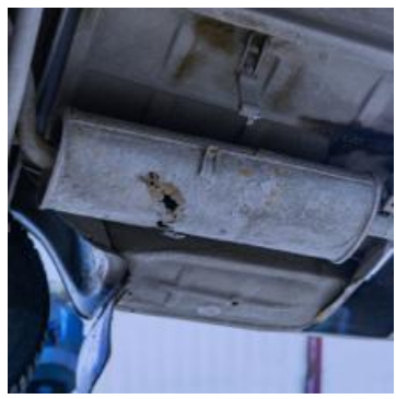
Image: An example of an old, rusted muffler that requires replacement.
