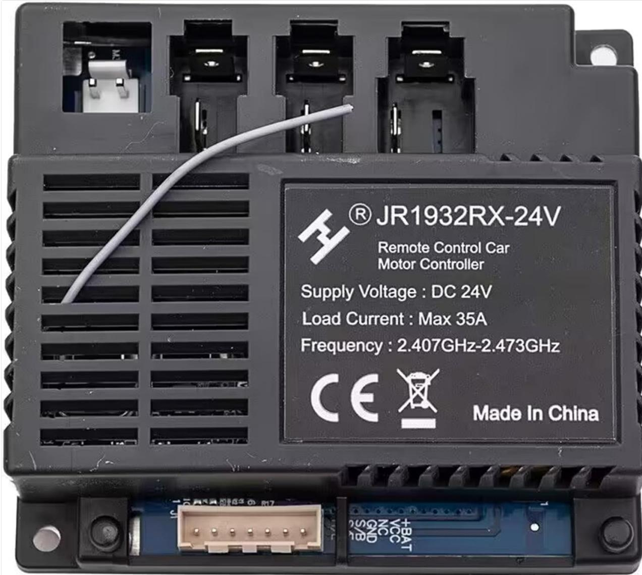
**Image Description:** This image displays the JR1932RX-24V 2.4G Receiver Control Box from a top-down perspective. The label clearly indicates 'JR1932RX-24V Remote Control Car Motor Controller', 'Supply Voltage: DC 24V', 'Load Current: Max 35A', and 'Frequency: 2.407GHz-2.473GHz'. Several connection ports are visible at the top, and a white antenna wire extends from the unit. The bottom edge shows a circuit board with a multi-pin connector.
