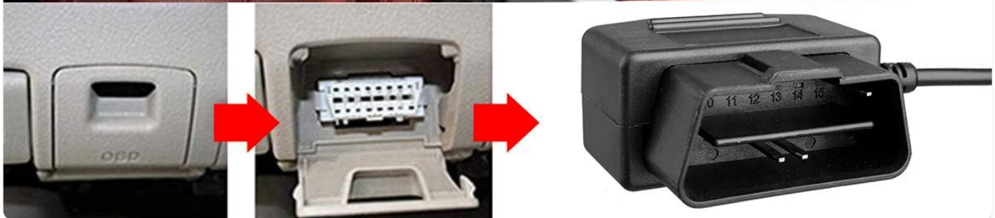
Image: Step-by-step guide for installing the OBD power cable, showing the OBD port location and connection to the dash cam.
