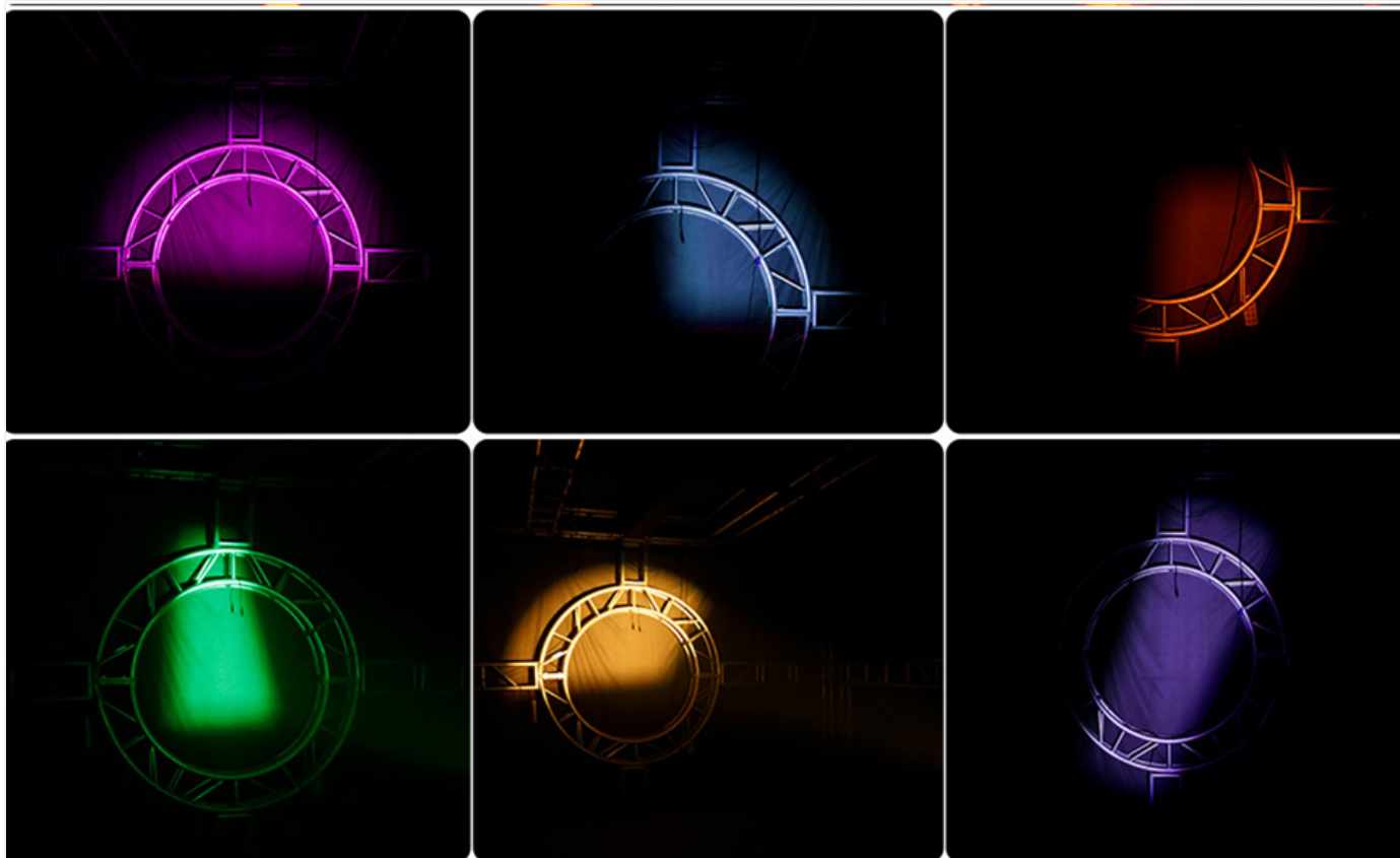
Figure 9: Examples of various light patterns that can be achieved with the adjustable shutters, including different shapes and partial projections.
