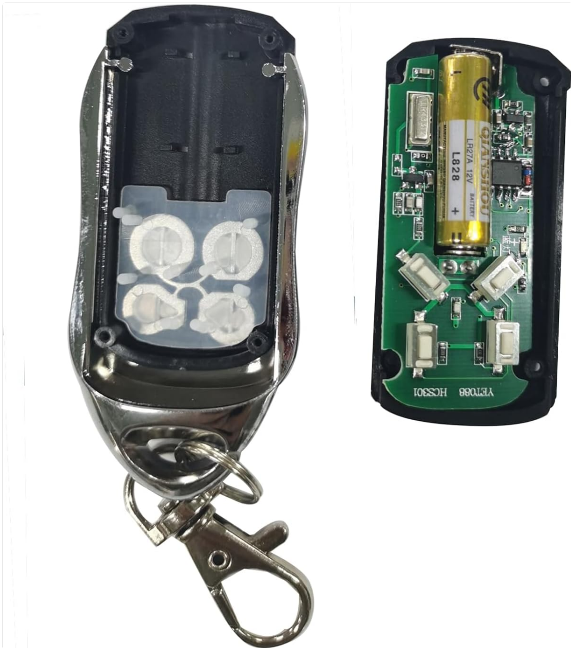
Image: Internal view of the RT77 remote control, showing the circuit board and the 12V 27A battery compartment.
