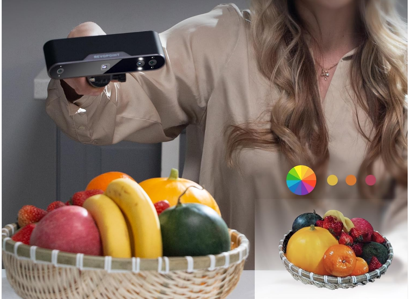
Figure 5: A basket of fruit being scanned by the Revopoint POP 3 3D Scanner, demonstrating its ability to capture lifelike color in 3D models.
