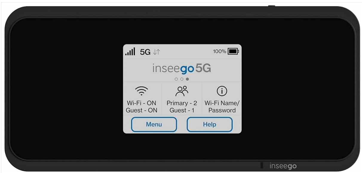
Figure 3.1: Front view of the Inseego MiFi M2000, showing the touchscreen display with network status, Wi-Fi status, and menu options.
