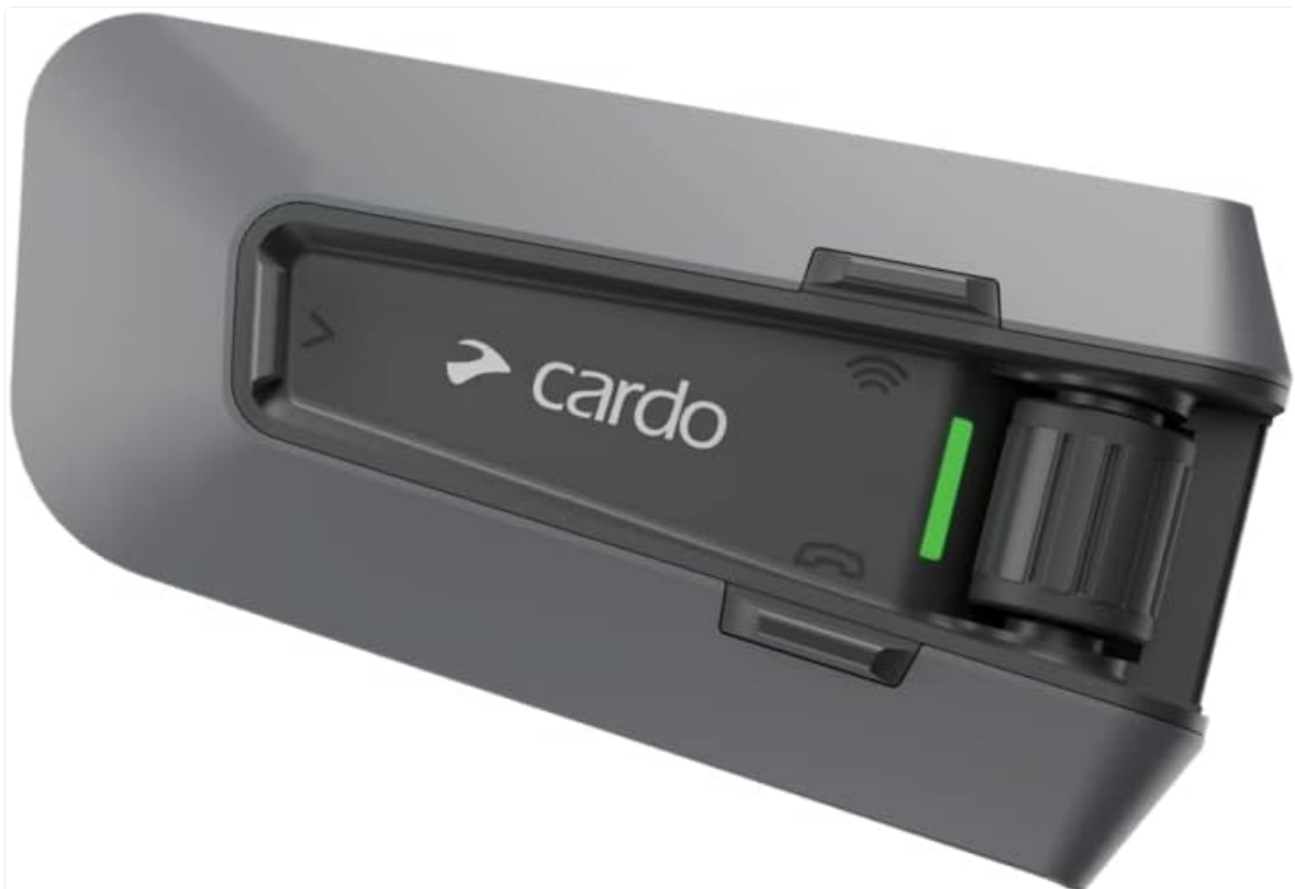
Figure 1: The Cardo PACKTALK Edge ORV communication unit, featuring a sleek design with a control roller and magnetic air mount.
