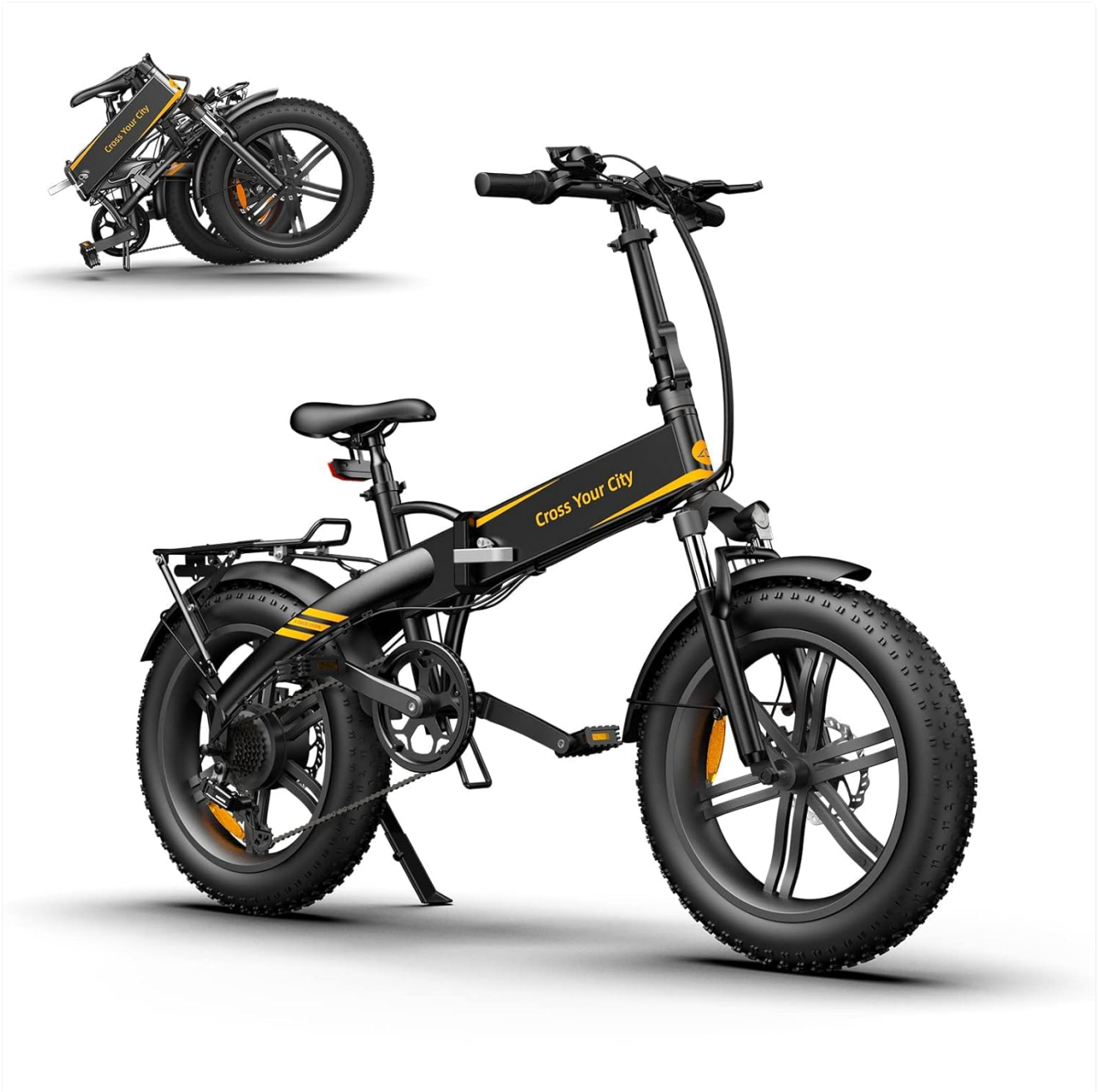
Figure 2.1: The ADO A20FXE electric bike shown in both its compact folded state and fully unfolded, ready for use.
