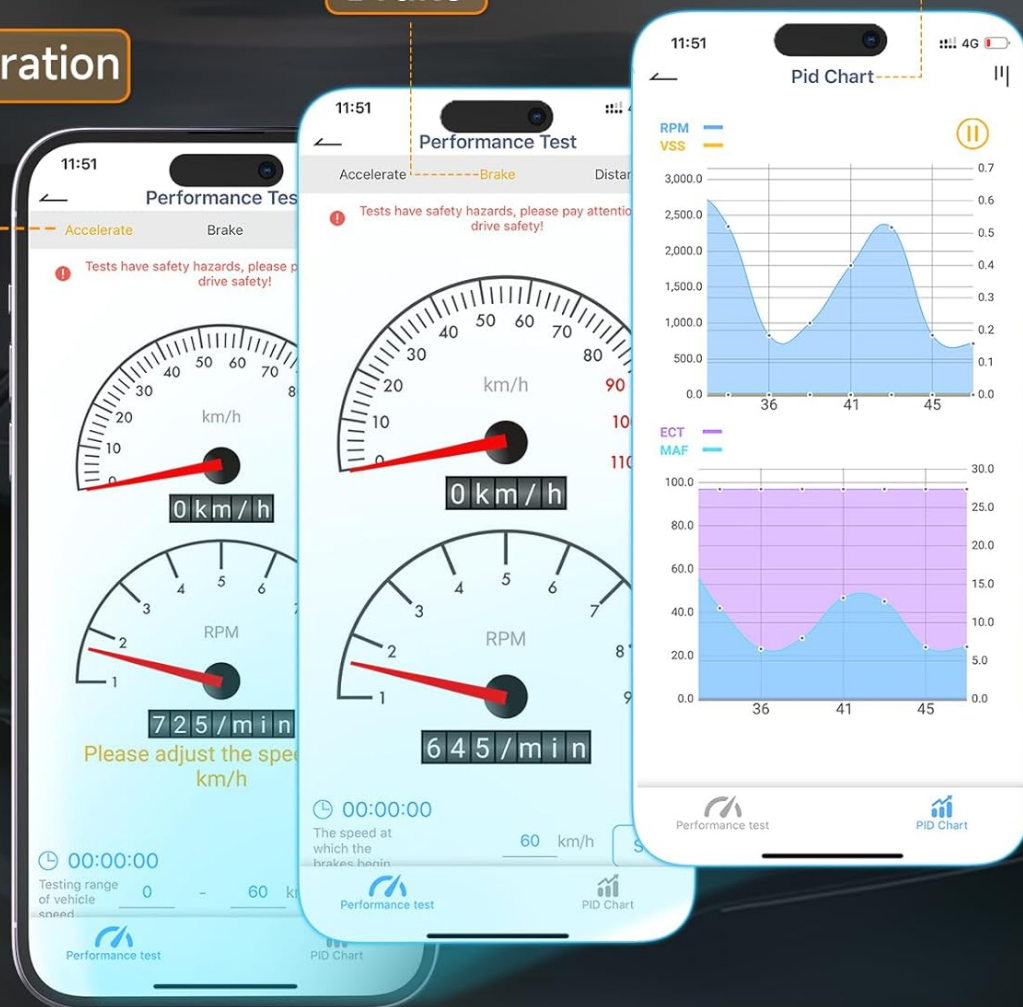
Image 5.1: The ANCEL app showing the Performance Test interface with acceleration and brake data.
