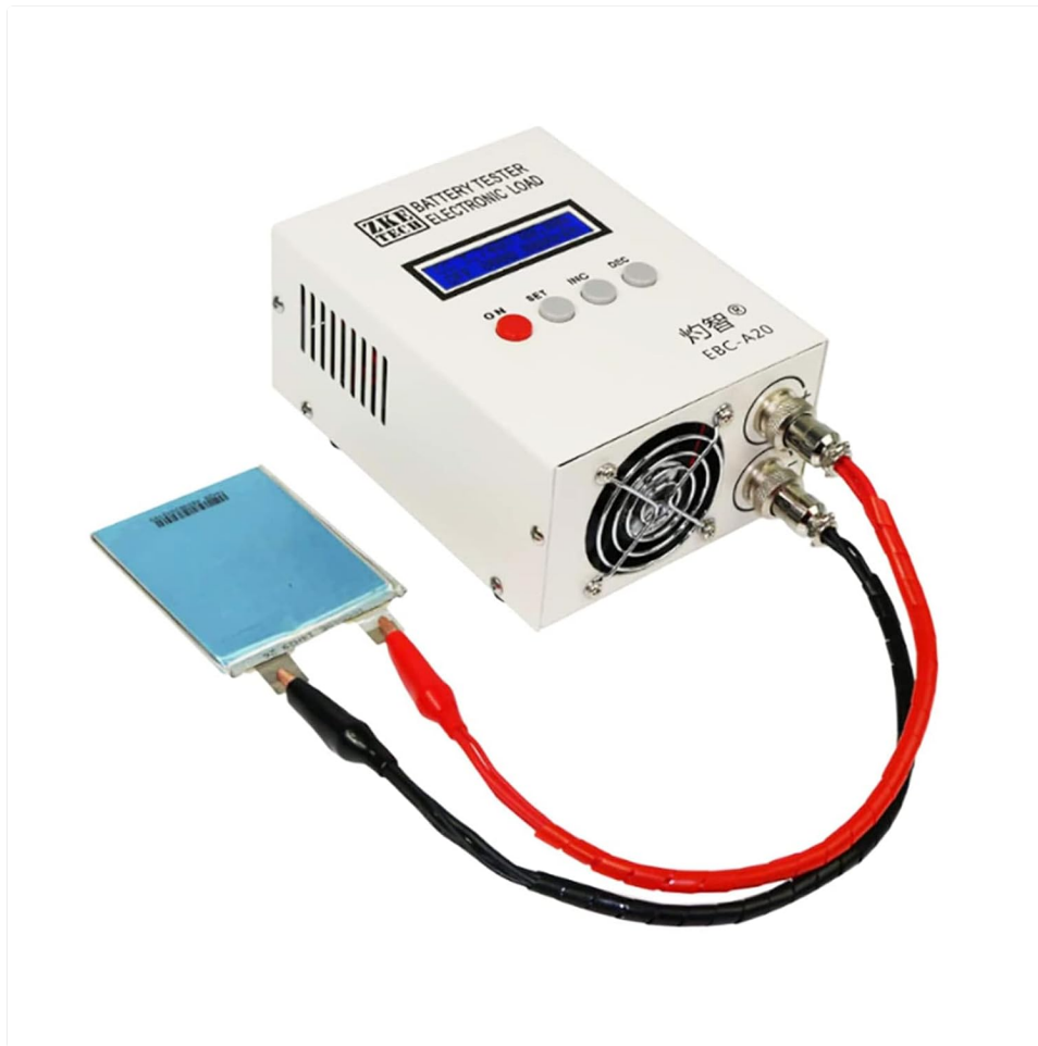
Figure 5.1: Proper 4-wire connection of a battery to the EBC-A20 for accurate testing.
