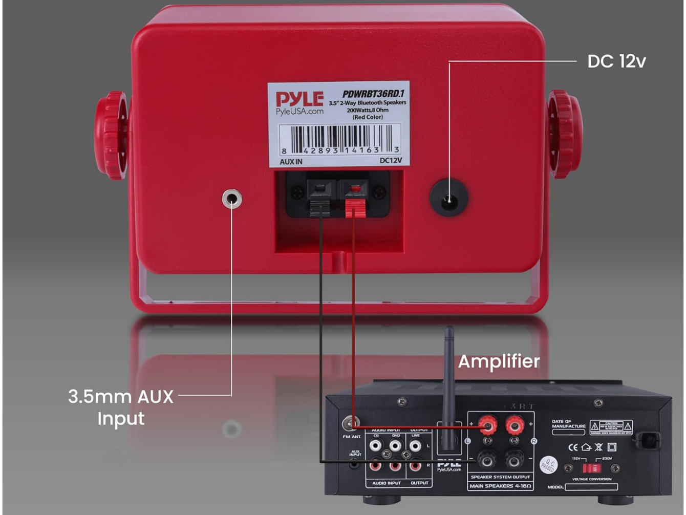
Image 3.2: Quick-Connect Terminals. The rear of the speaker shows the quick-connect terminals for speaker wire, the DC 12V power input, and a 3.5mm AUX input.
