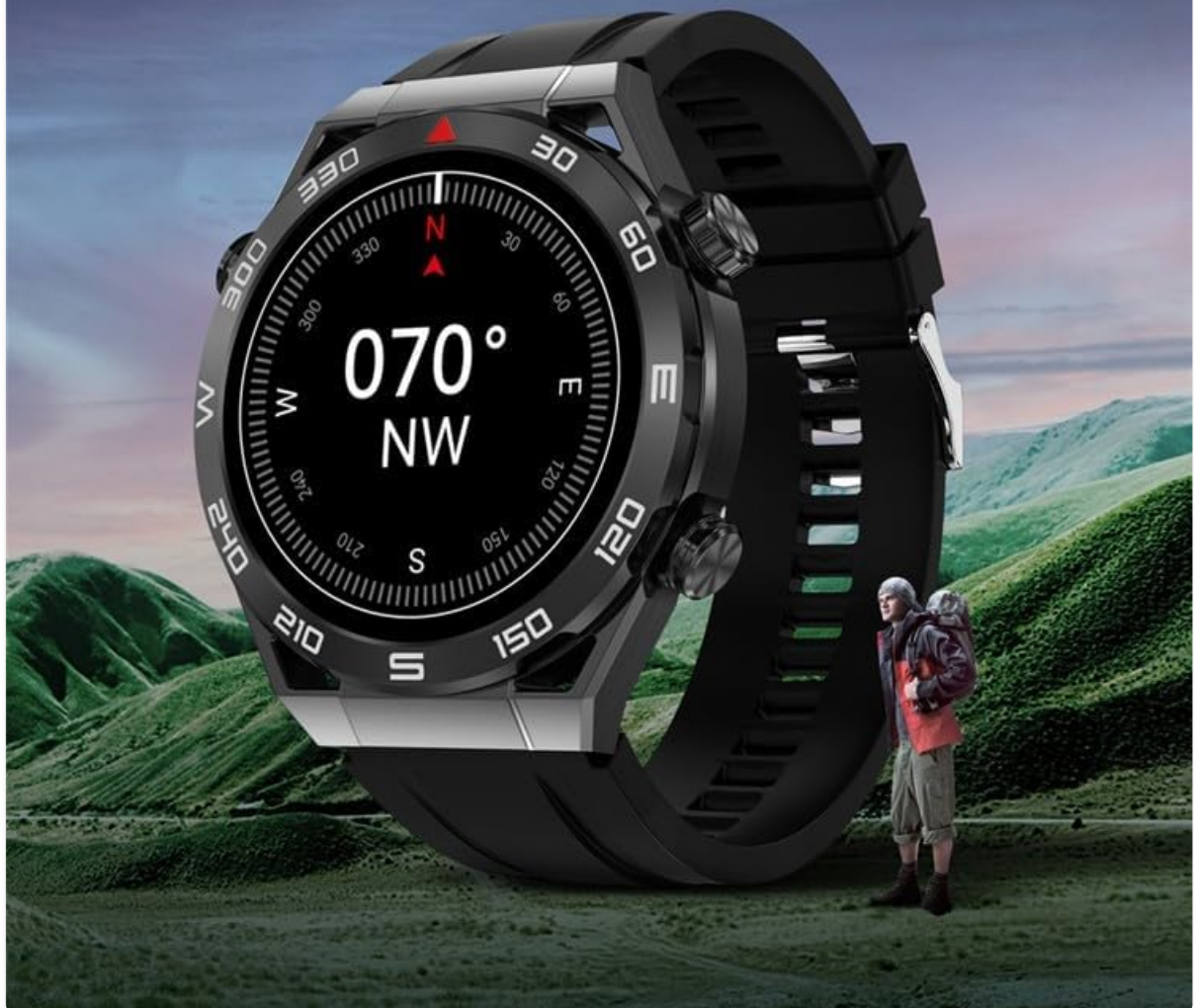
The smartwatch displaying its built-in digital compass, indicating direction and degrees.
