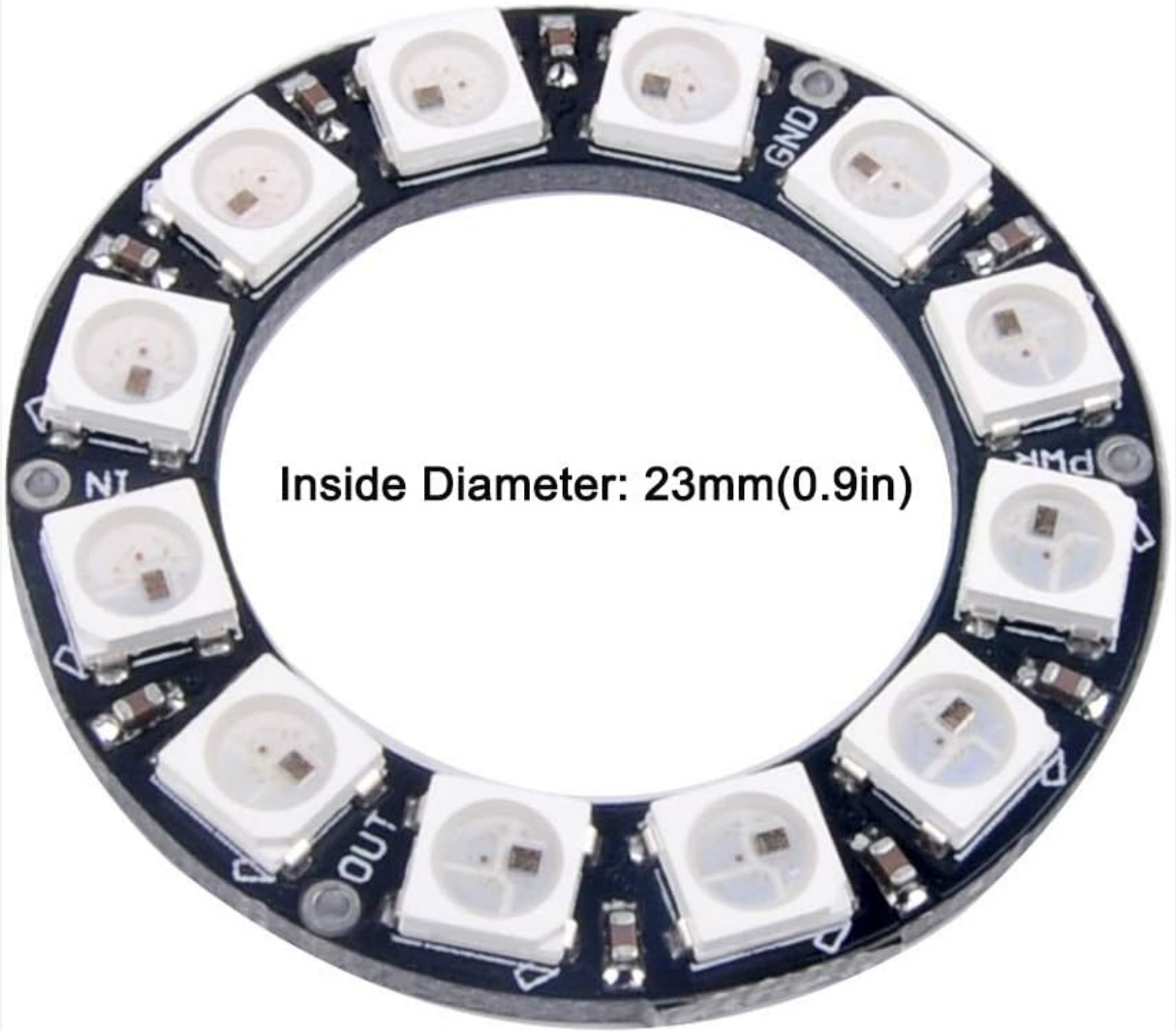
Image: A close-up view of the LED ring showing its dimensions: Outside Diameter: 37mm (1.45in), Inside Diameter: 23mm (0.9in).
