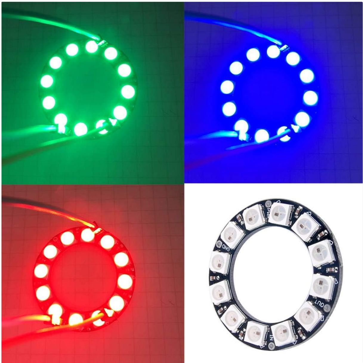
Image: Multiple WS2812B RGB LED rings illuminated in green, blue, and red, demonstrating their full-color capabilities.
