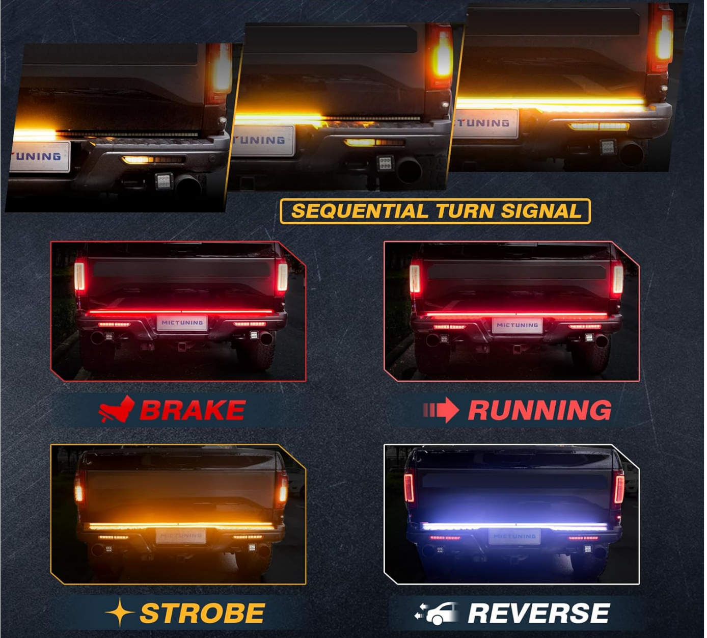
Figure 3: Illustration of the five distinct lighting modes: Sequential Turn Signal, Strobe, Brake, Running, and Reverse.
