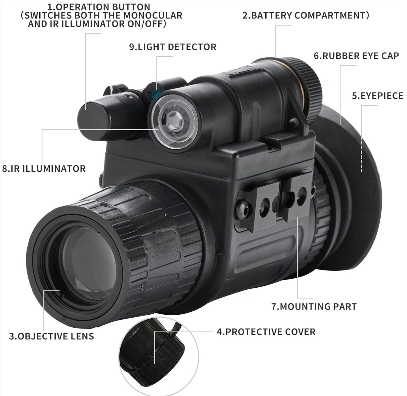
Figure 1: Labeled components of the PVS 14 Monocular.
