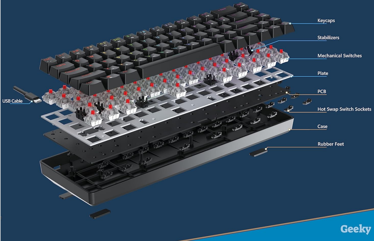
Figure 3.3: Exploded view illustrating the internal structure of the GK65, from keycaps to the base case.
