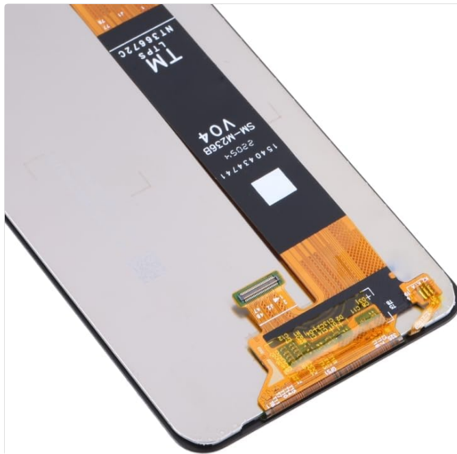
Image 5.2: A detailed close-up of the flex cable connector on the replacement screen assembly, which connects to the phone's motherboard for display and touch functionality.
