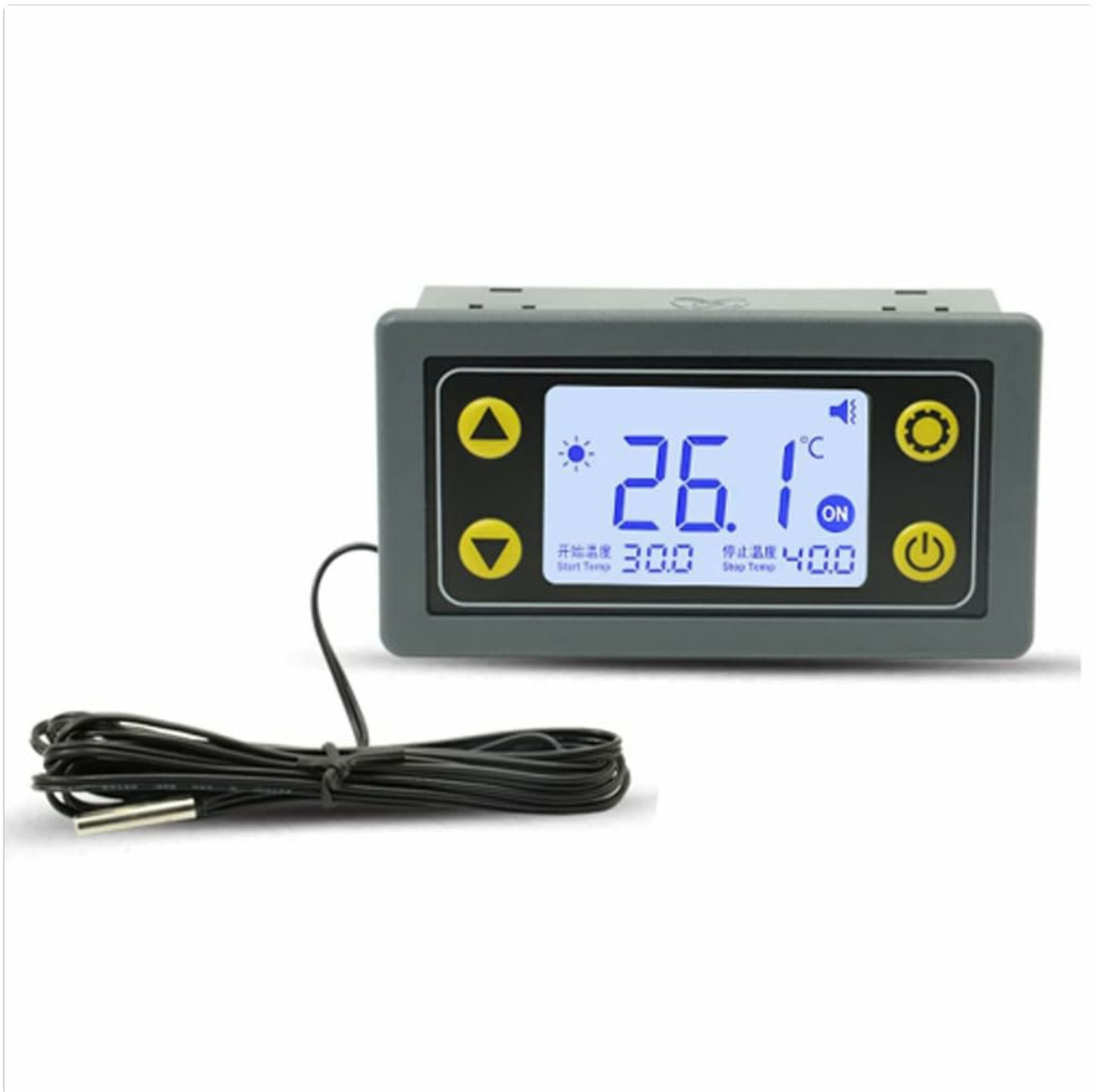
Figure 2.1: Senzooe XY-ST10 Temperature Controller Module. The module features a digital display showing the current temperature (26.1°C), set start temperature (30.0), and set stop temperature (40.0). Control buttons include Up, Down, Set (gear icon), and Power. A wired temperature probe is connected to the unit.
