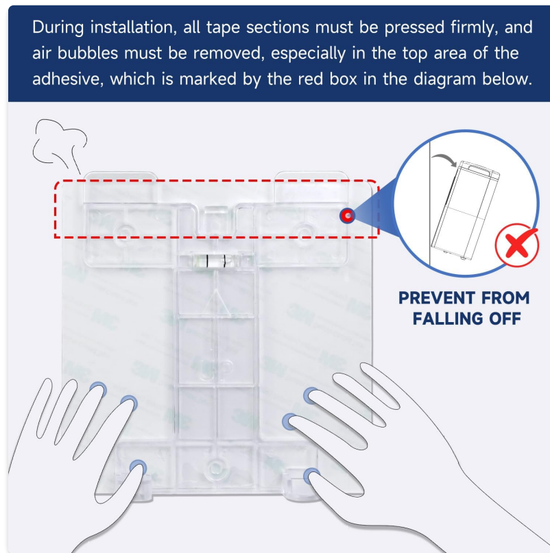
Figure 3: Proper technique for pressing the adhesive mounting plate during installation.
