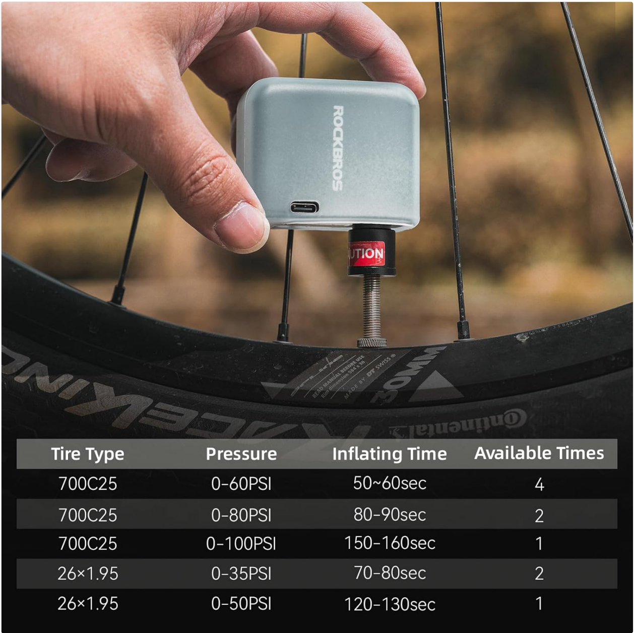
Image: A table detailing the pump's performance, including tire type, target pressure, inflation time, and number of inflations per full charge.
