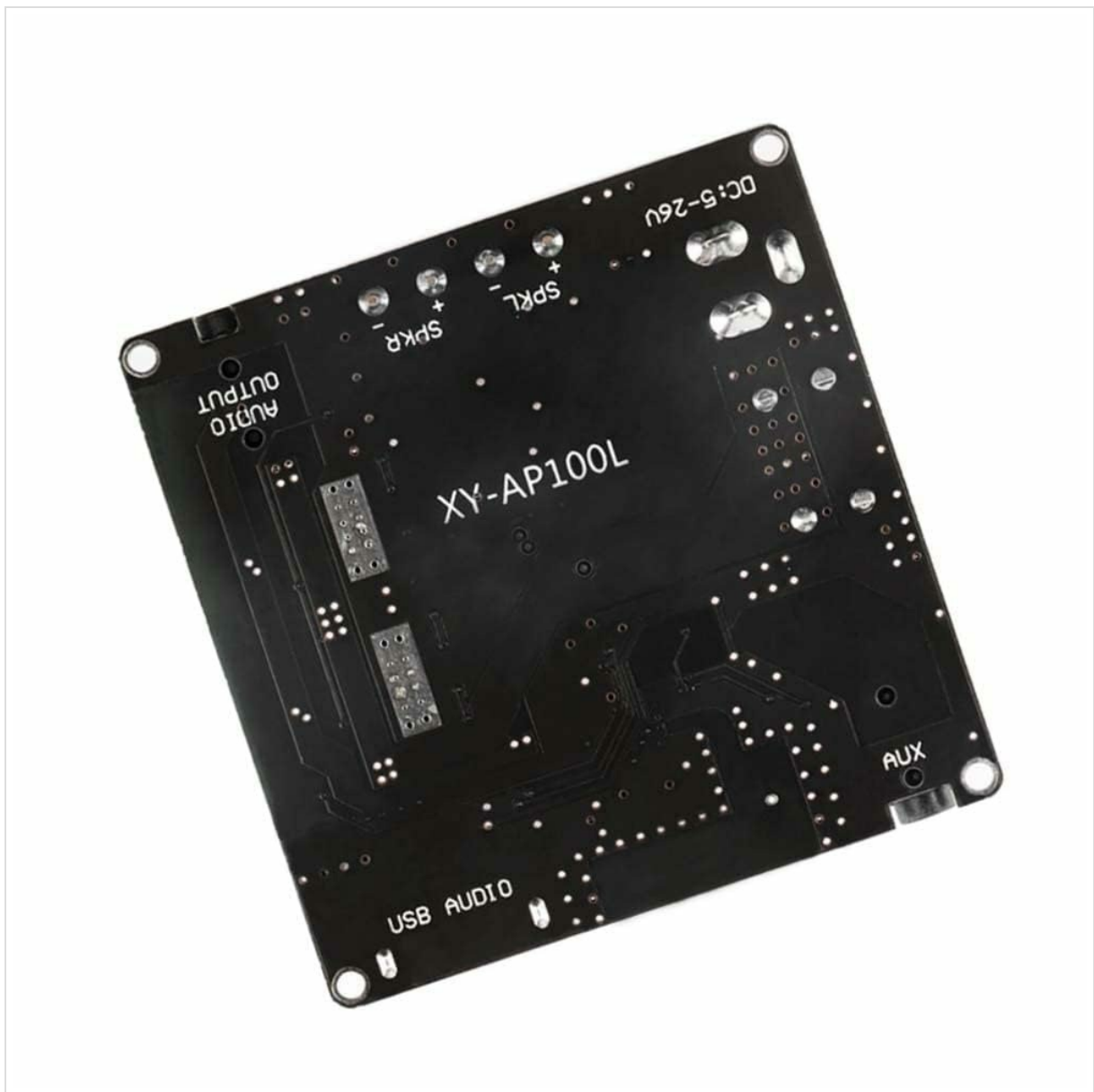
Figure 2: Bottom View of Amplifier Board. This image shows the underside of the XY-AP100L amplifier board, revealing the printed circuit board (PCB) traces, solder points, and various surface-mount components. Labels for speaker outputs (SPKR L, SPKR R), DC 5-24V, AUX, and USB AUDIO are also visible from this perspective.
