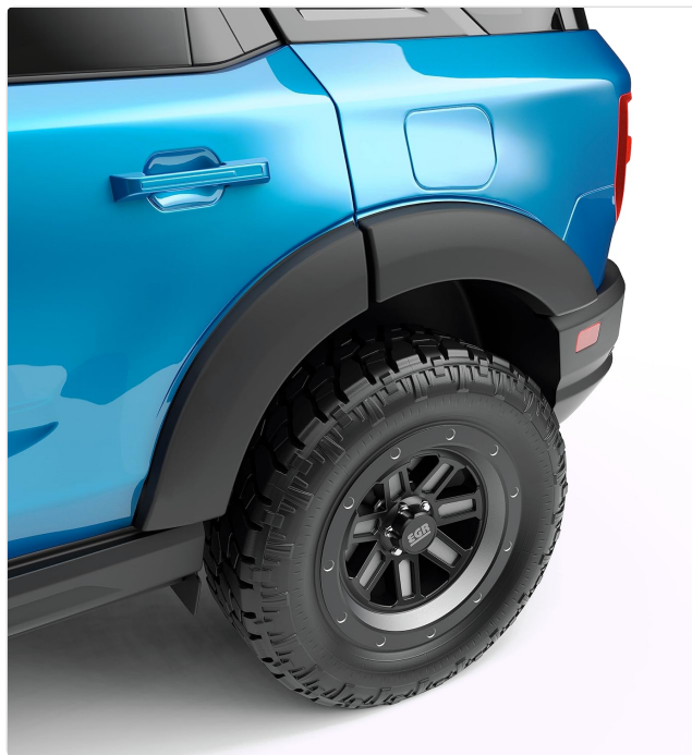
Figure 4: Detailed view of the rear fender flare, showing its integration with the vehicle's body.
