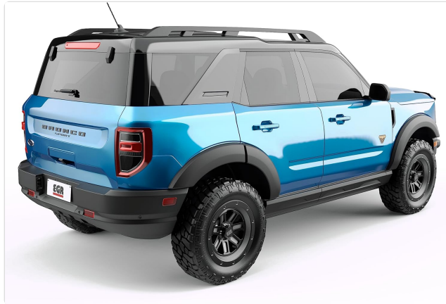
Figure 6: Rear perspective showing the extended tire coverage provided by the fender flares.
