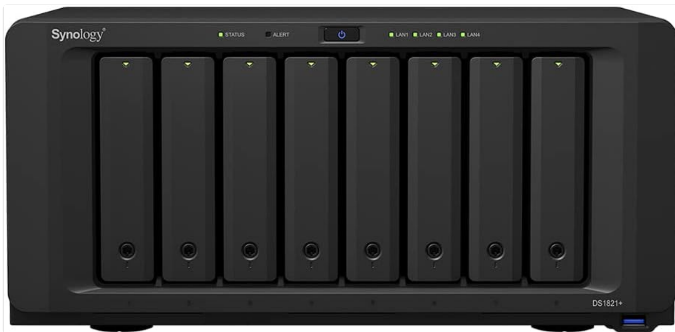
Figure 1: Front view of the Synology DS1821+ DiskStation, showing the eight accessible drive bays, status indicators, and power button.
