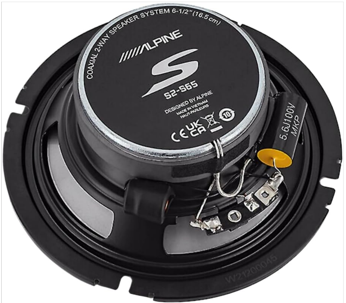
Figure 2: Rear view of the Alpine S2-S65 speaker, highlighting wiring terminals.
