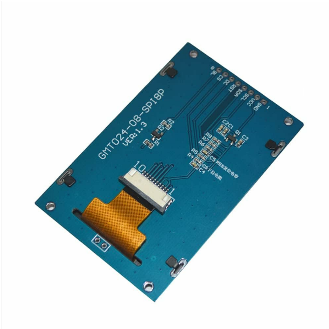
Figure 4.1: Rear view of the Senzooe 2.4 inch IPS LCD module, highlighting the pin header for electrical connections and the integrated circuit board.
