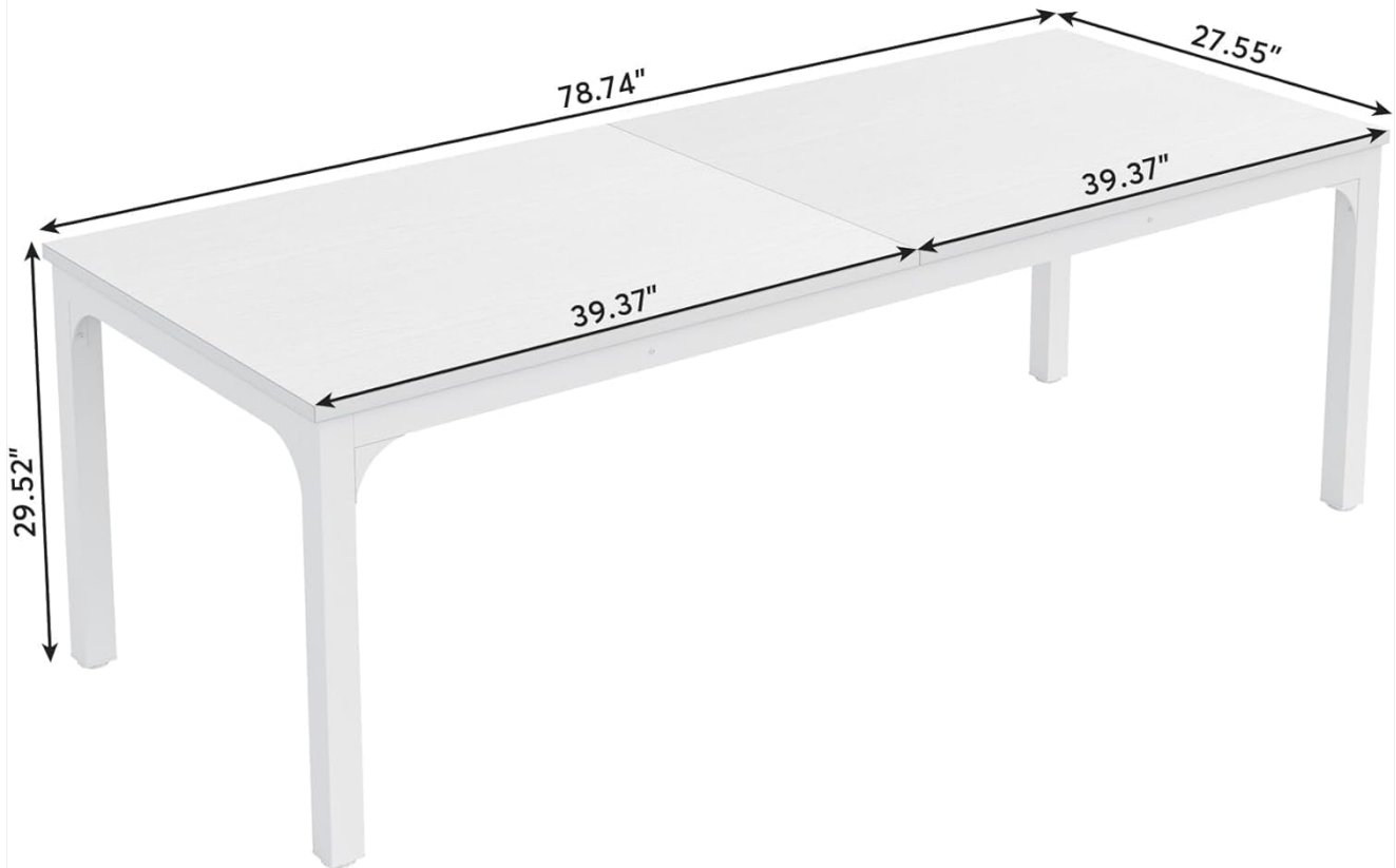
Image 2: Dimensional diagram of the desk, indicating its overall length, width, and height.
