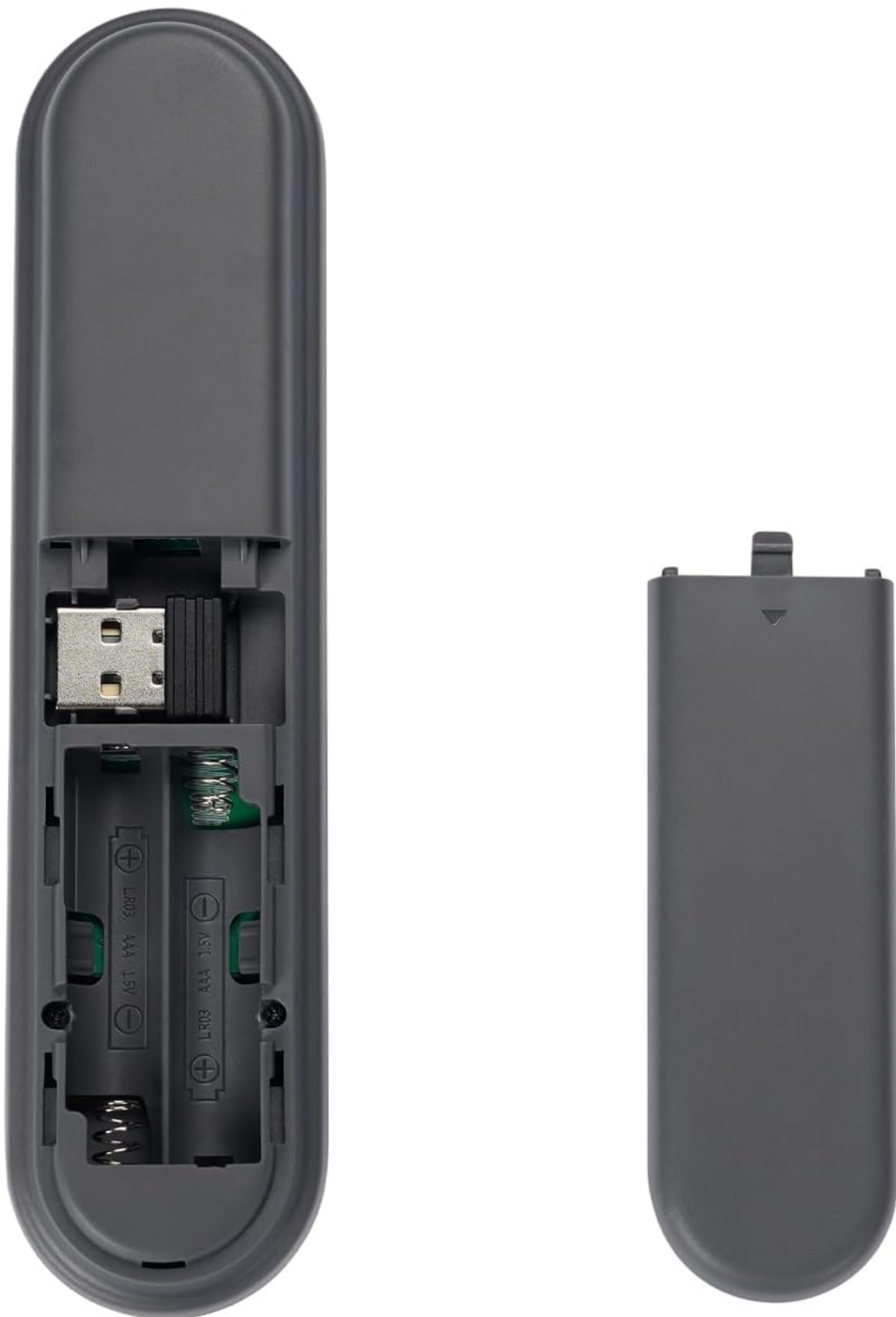
Image: Rear view of the remote control showing the battery compartment and the USB receiver slot.
